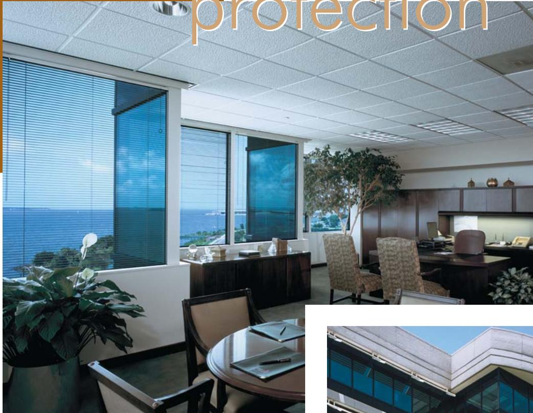
Vista® UVShield® Nuance film was selected and installed on over 900 windows, 25,000 square feet of glass in all. The Vista® film blocks almost all (99.9%) of the sun's ultraviolet rays at the glass surface and reduces the sun's glare by half (48%) without impairing the scenic views day or night. Furthermore, with harsh glare gone, computer screens no longer need to be sheltered to be read, meaning that work can be accomplished and views enjoyed simultaneously.
